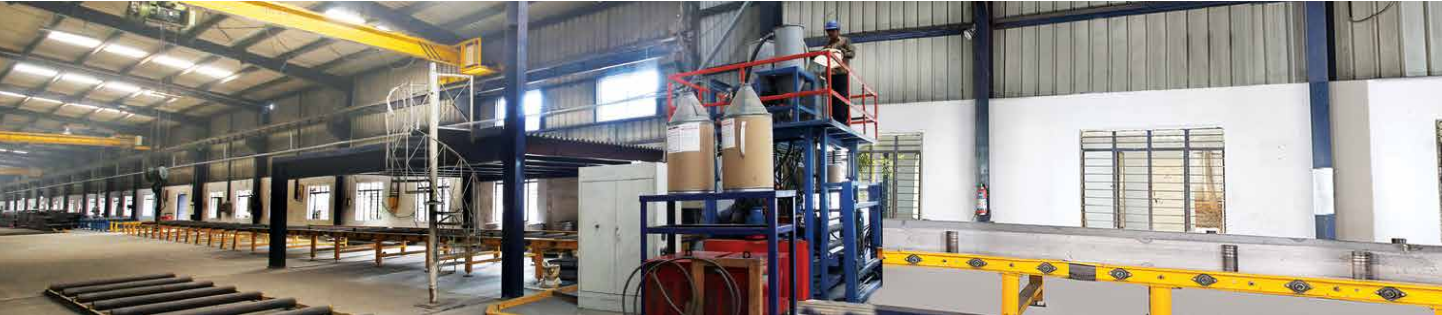
H - BEAM SAW WELDING MACHINE
